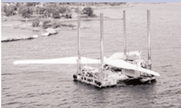
Figure 1.24: Blade Handling for Transport by Sea
