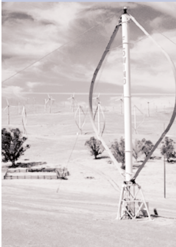
Figure 1.2: Darreius Type Vertical Axis Wind Turbine
